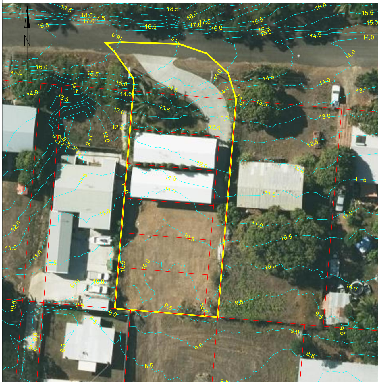
LIDAR CONTOURS - LIDAR DATA FROM 2011 (PRE SITE DEVELOPMENT) AERIAL IMAGERY FROM 2021 CONTOURS AT 0.5m SPACINGS
