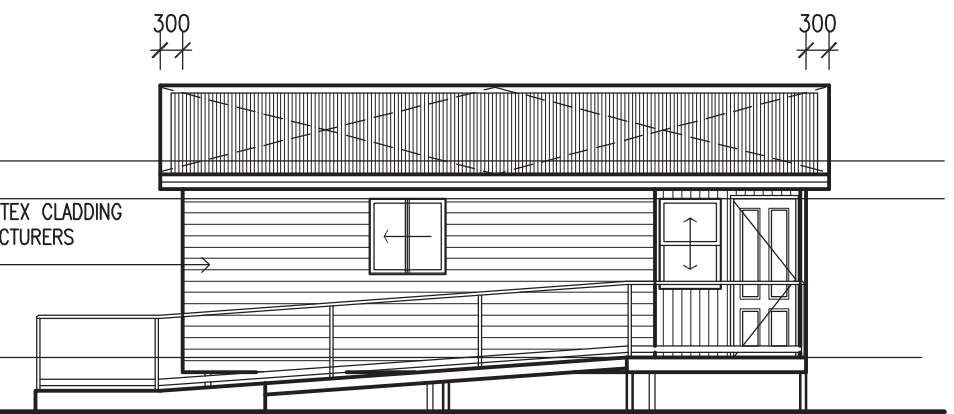
SIDE ELEVATION (CARETAKERS ACCOM/OFFICE) 1:100
